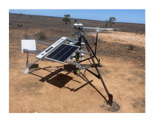
The Solar Monitoring Station is an autonomous tripod-mounted data logger system, providing reliable data collection for solar resource measurements.
