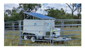
The robust A-frame mounted deployment box means that your WindCube® v2.1 will travel to site safely and securely, removing the need for onsite installation or lifting.
